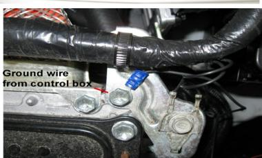
Sensor and buzzer connections made into Control Box. Ground connection made. Control Box is mounted on top of fuse box with supplied adhesive tape.
