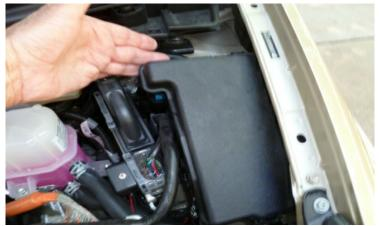
Power fuse tap inserted in fuse box. Thin red power wire is brought out of front of fuse box and fuse box cover is snapped into place. If you use the fuse tap in a different fuse location, use the removed fuse in the lower fuse tap holder to maintain that function.
