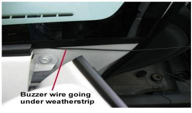
Buzzer wire hidden under the top weatherstripping
