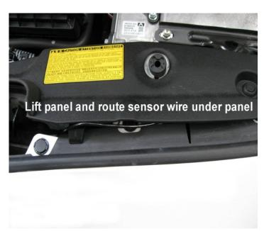
Route the sensor cable under the plastic panel as shown. Push down panel into original position.
